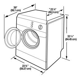
\*Most installations require a minimum 5½" (14.0 cm) clearance behind the dryer for the exhaust vent with elbows. See "Venting Requirements."
